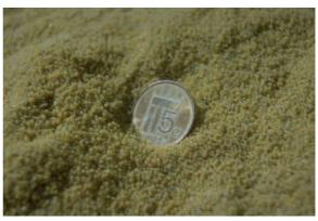
Figure 3 - Limestone pellets
